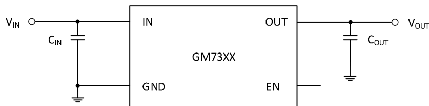
Typical Application Circuit
