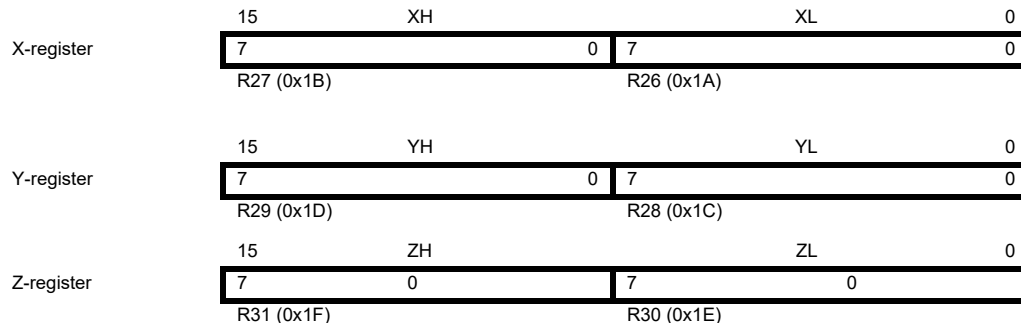
Figure 7-3. The X-, Y-, and Z-registers
